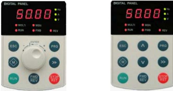
Note: 5.5 kW and below standard for shuttle type operation panel (IE knob type), 7.5 kW and above for Key-type operation panel. If the customer needs to change the operation panel, please specify when ordering.
