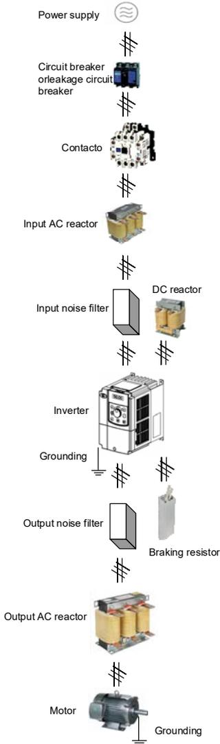
Fig.2-1 Connection diagram of the product and peripheral devices
