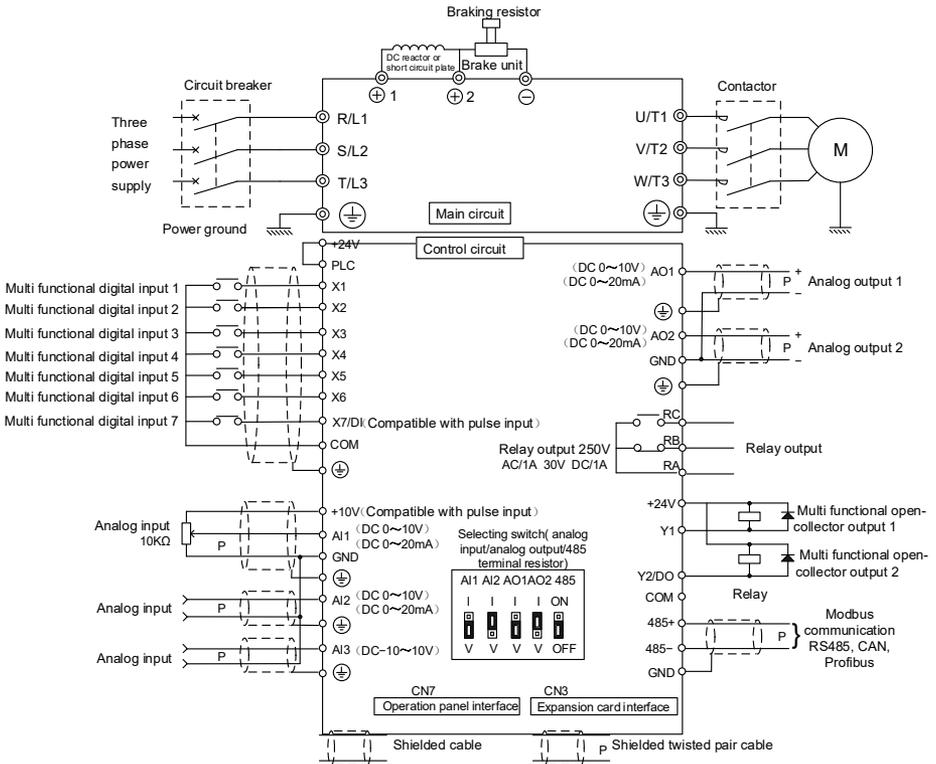
Figure 2-2 Terminal wiring diagram
